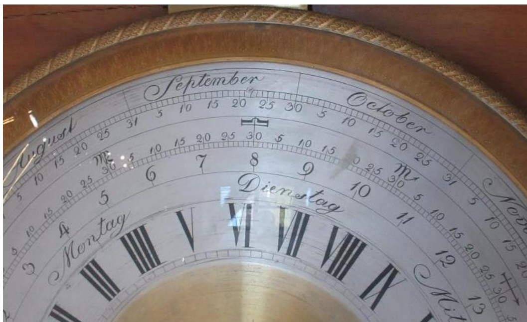
Figure 7.25: Hahn's Weltmaschine : detail of the middle central dial giving the day of the week and the month. (photograph by the author, 2025)
