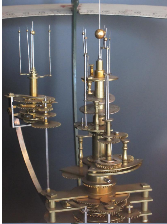
Figure 7.18: Hahn's Weltmaschine : the central part of the orrery and the system of Jupiter. (photograph by the author, 2025)
