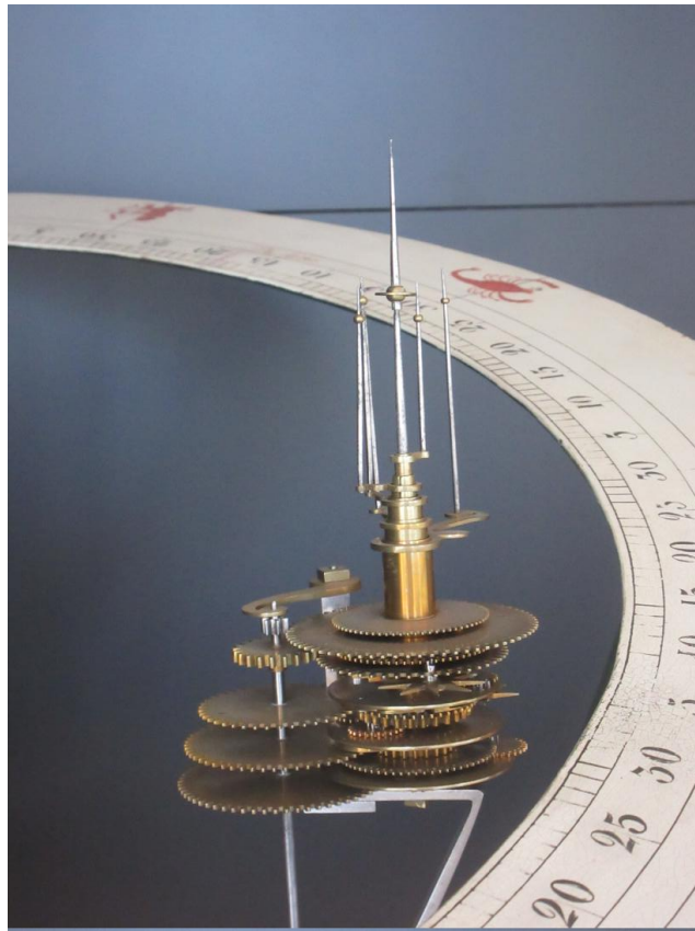
Figure 7.21: Hahn’s Weltmaschine : detail of the system of Saturn. (photograph by the author, 2025)
