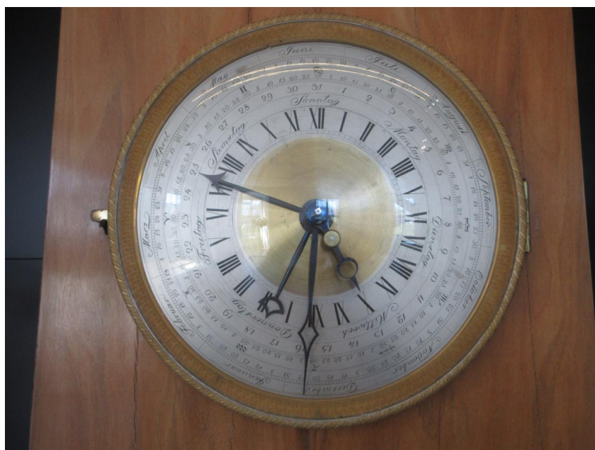
Figure 7.24: Hahn's Weltmaschine : the middle central dial giving the day of the week and the month. (photograph by the author, 2025)
