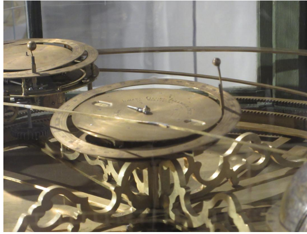
Figure 6.6: The central part of Frater Fridericus's clock in Bamberg, with the motion of Mercury. The tilted ring causes Mercury to move up and down. (photograph by the author)
