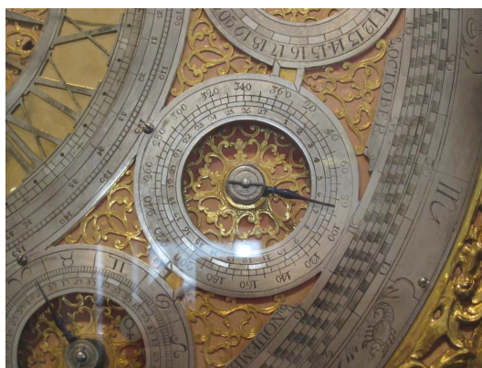
Figure 4.18: The dial for the anomalistic month on Frater David's clock. (photograph by the author)
