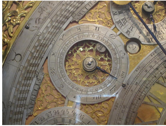
Figure 4.14: The dial for the tropical motion of Jupiter on Frater David's clock. (photograph by the author)
