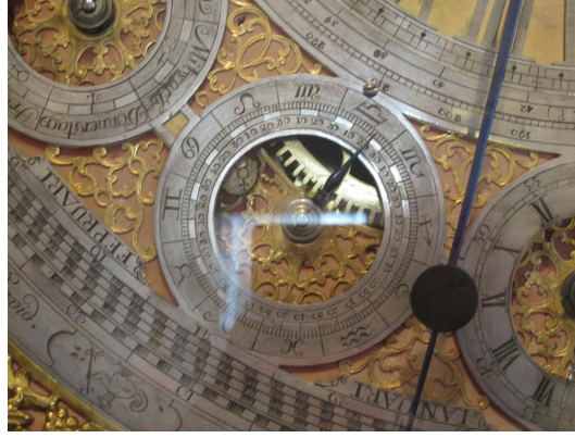
Figure 4.11: The dial for the tropical motion of Mercury on Frater David's clock. (photograph by the author)
