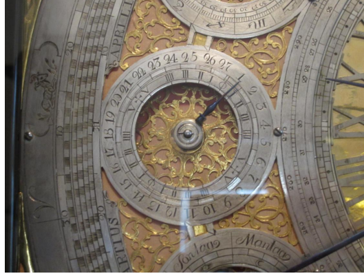
Figure 4.16: The dial for the draconic month on Frater David's clock. (photograph by the author)
