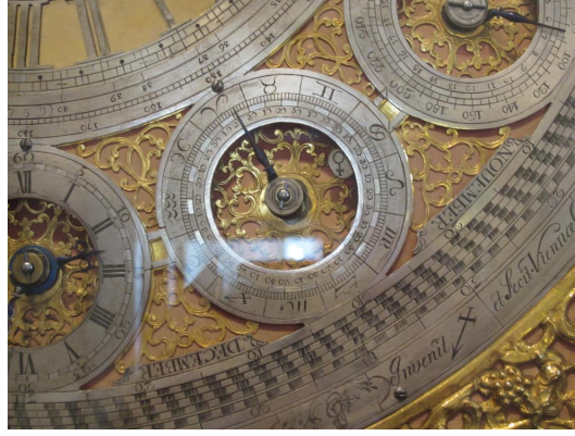
Figure 4.12: The dial for the tropical motion of Venus on Frater David's clock. (photograph by the author)
