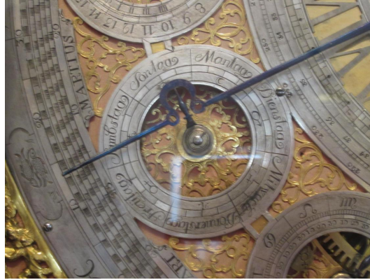
Figure 4.10: The dial for the day of the week on Frater David's clock. (photograph by the author)
