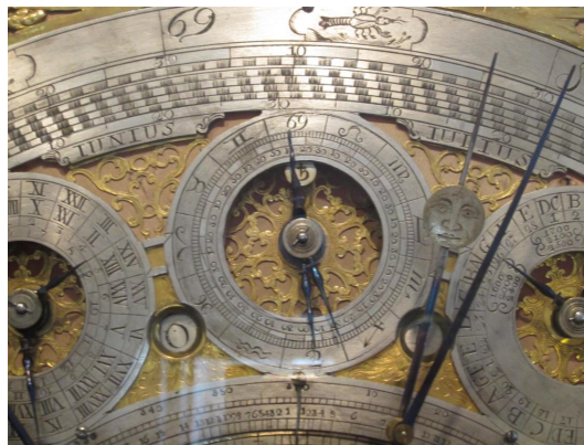
Figure 4.15: The dial for the tropical motion of Saturn as well as the prograde motion of the Earth's perihelion on Frater David's clock. (photograph by the author)
