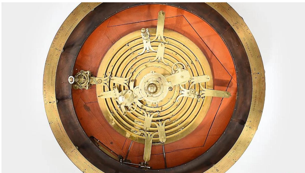
Figure 2.7: The large driving wheels of Adams' orrery, when the top cover is removed. Saturn is visible on the left. (excerpt from the video https://www.youtube.com/watch?v=0L3G-1VG7Mw )
