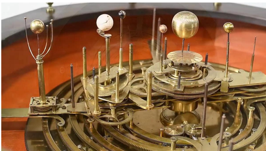
Figure 2.8: From left to right, the gears for Jupiter, the Earth/Moon system, Mercury and Venus in Adams' orrery. (excerpt from the video https://www.youtube.com/watch?v=0L3G-1VG7Mw )
