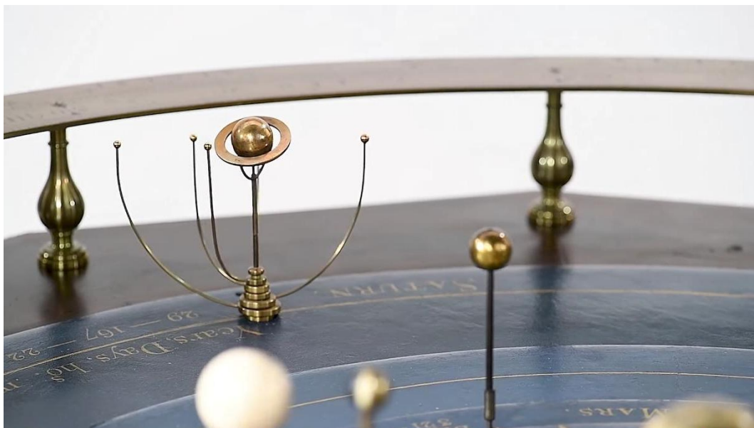
Figure 2.15: Saturn and its satellites when the top cover of Adams' orrery conceals the gears. (excerpt from the video https://www.youtube.com/watch?v=OL3G-1VG7Mw )
